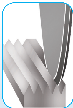
The inserts are ground to create sharp grooves.
